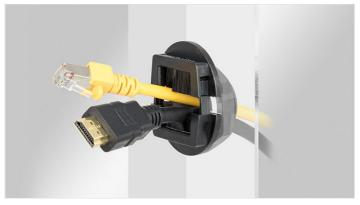
For round metric cut-outs M32/M50 icotek offers the split cable gland with brush strips KEL-BES-S round. It can be either directly snapped into the cut-out or screwed with a locknut, which is included in the shipment.
